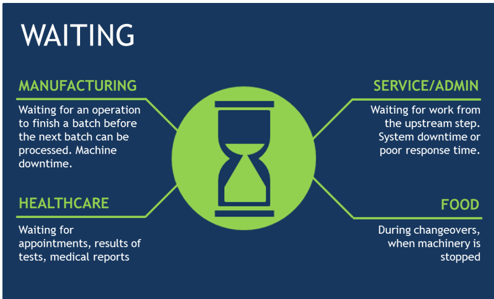
Figure 12 Examples of the waste of WAITING
